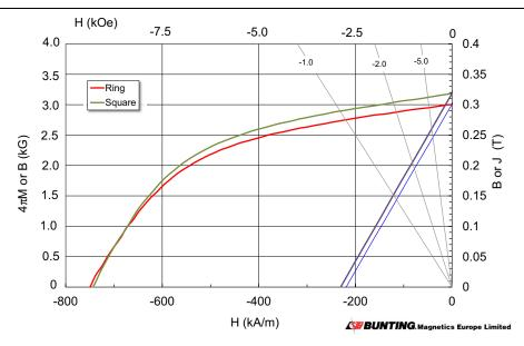
Fig. 5. Hysteresis loops of the binder jet printed ring and square magnets.
