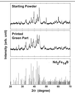
Fig. 2. XRD patterns of as-received MQP powders (top) and binder jet printed magnet part (center). The vertical lines indicate the peak positions for  $Nd_2Fe_{14}B$  phase (bottom).
