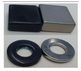
Fig. 1. Images of 1"  $\times$  1" square (2.54  $\times$  2.54 cm) and 1" (2.54 cm) ring near-net-shape binder jet magnets after a clear polyurethane coat compared with nickel-coated commercially sintered NdFeB magnets.
