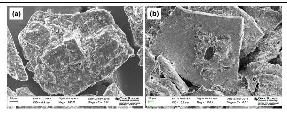
Fig. 3. SEM images of (a) as-received commercial MQP powders, and (b) binder jet printed magnet part.
